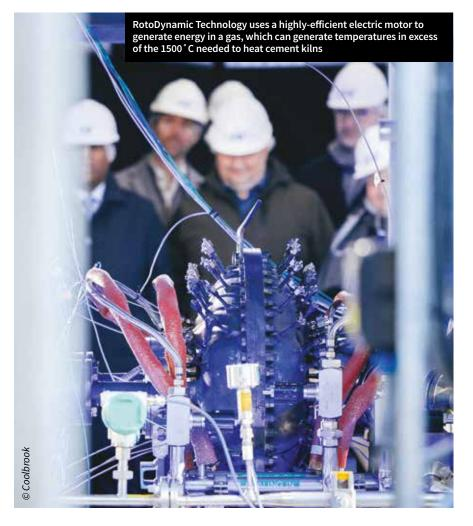
turbine, a highly-efficient electric motor spins blades to generate energy in the gas, which is expressed through heat.
